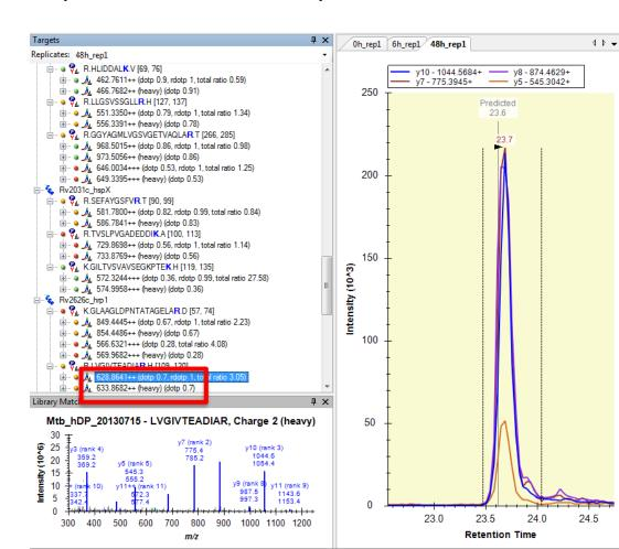
We can use a synthetic standard to generate a reference spectrum for the spectral library in SRM:
