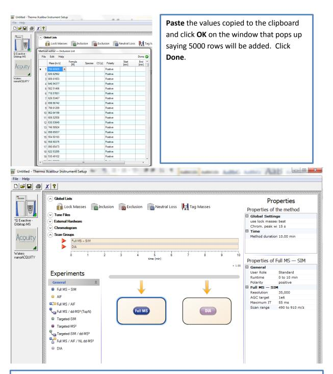
Add a **Full MS-SIM** and **DIA** scan event to the method. This is done by clicking and dragging the scan event name from the list of **Experiments** and dropping the event onto the grey timeline bar just to the right of where it says **Experiments**. Click the **Full MS** scan event that was just dragged over. The properties that I use for this scan event are displayed on the right.
