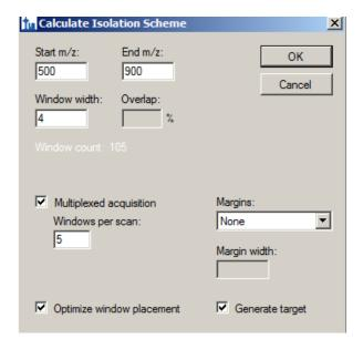
Enter 500 as the Start m/z and 900 as the End m/z. Window width should be 4. Selecte Multiplexed acquisition with 5 windows per scan. Select Optimize window placement and Generate target. Click OK.
