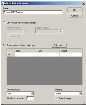
Enter a name for the isolation scheme in the box that says Name, select Prespecified isolation windows, under Deconvolution select Msx and in Windows per scan enter 5. Select Specify target and click Calculate...
