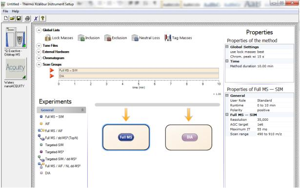
Add a **Full MS-SIM** and **DIA** scan event to the method. This is done by clicking and dragging the scan event name from the list of **Experiments** and dropping the event onto the grey timeline bar just to the right of where it says **Experiments**. Click the **Full MS** scan event that was just dragged over. The properties that I use for this scan event are displayed on the right.
