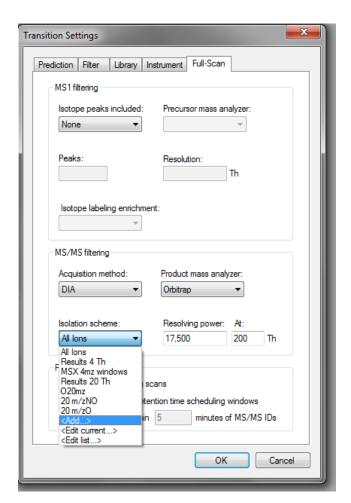
Click on the Full-Scan tab, set Acquisition Method to DIA, Product mass analyzer to Orbitrap, and under Isolation scheme click <Add...>
