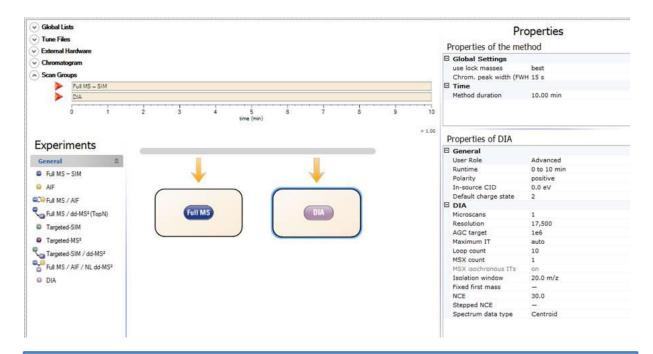
Click on the **DIA** scan. The properties that I use are shown on the right. The **Loop Count** of 10 means that an MS scan will be taken every 10 MS/MS (DIA) scans.
