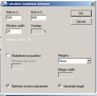
Enter a start m/z and end m/z for the precursor m/z range you would like to analyze by DIA. I use 500 - 900 with a Window width: of  $20 \ m/z$ . Click the checkbox for Optimize window placement, and Generate target. Optimize window placement avoids placing edges of the isolation windows in regions where peptides are likely to occur. Generate target causes Skyline to output the center of each isolation window along with the start and end. Click OK.
